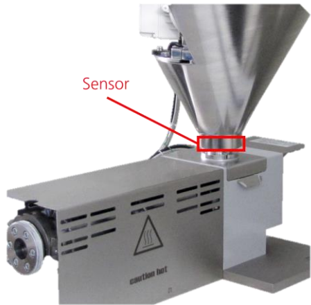
Monitoring of raw materials in dosing zone by eddy current and ultrasonics
